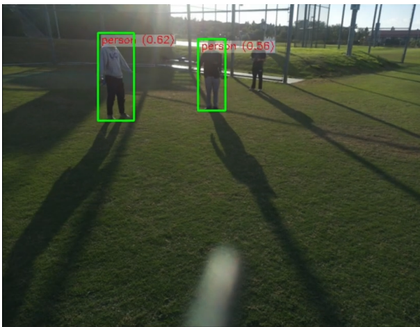
Fig. 15. Object detection stream screenshot while drone is flying
