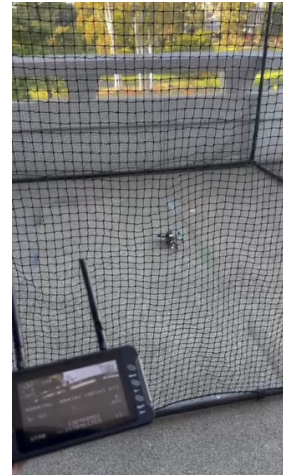
Fig. 9. Drone in cage, engaging motors and FPV camera feed
